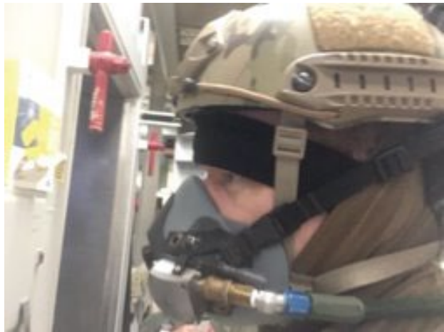
Figure 6: PSM headband being tested in a simulated low-pressure environment Credit: AFFOA
